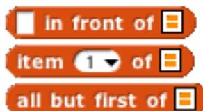
In a functional program, we often use recursion to construct a list, one item at a time. The **in front of** block makes a list that has one item added to the front of an existing list, *without changing the value of the original list*. A nonempty list is processed by dividing it into its first item (**item 1 of**) and all the rest of the items (**all but first of**), which are handled through a recursive call:
